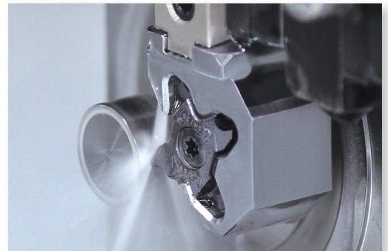
All cutting heads are available with high pressure through-coolant supply
